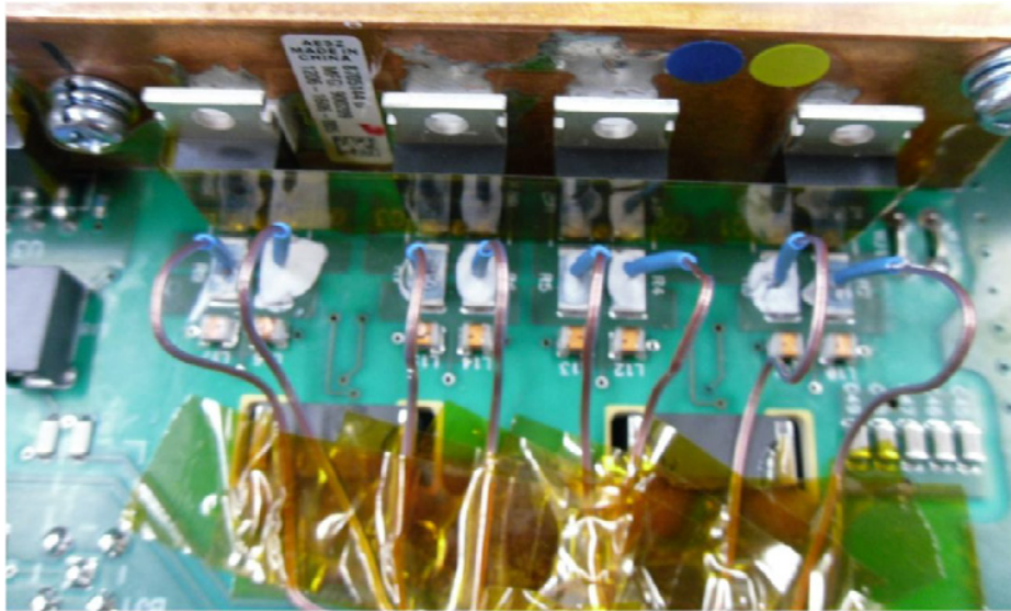
Figure 9: thermocouple placement on gate drive resistors.
