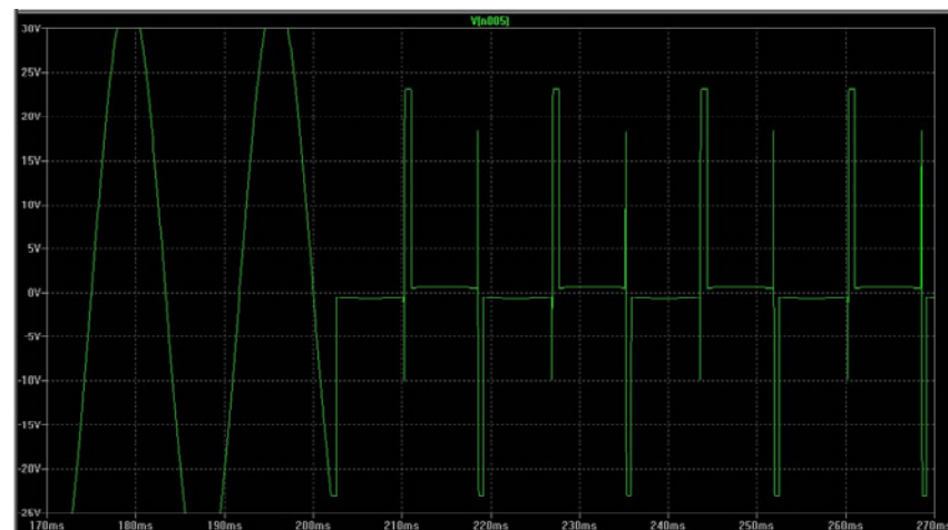
Figure 11 : Variable TRIAC, gate current 16.9mA. (close-up of turn-on characteristics)
