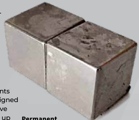
Permanent magnet cubes used in levitation systems on the Nevomo demonstration vehicle
