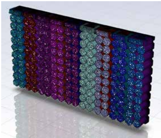
Volumetric meshing of battery pack to power electric airplane Image courtesy of Nordic Air Racing
