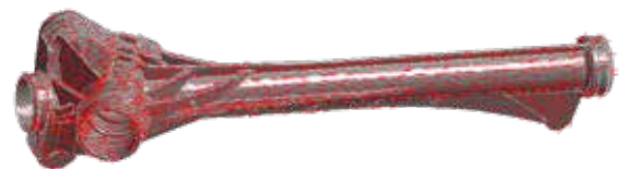
Figure 3. The main fiber directions are shown in red, mapped to the meshed geometry of the plastic housing using the orientation tensor in output from the injection molding simulation.
