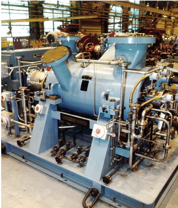
▲ Industrial centrifugal compressor COURTESY DRESSER-RAND.
