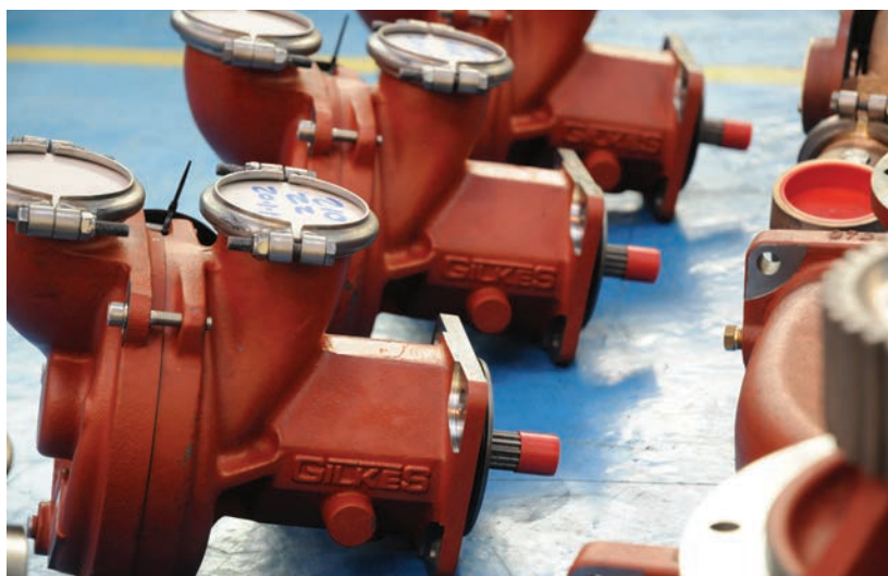
▲ Gilkes cooling pumps
