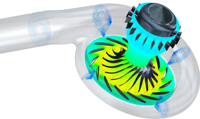
▲ 3-D flow simulation using ANSYS CFD allowed Continental Industrie to improve the performance of a centrifugal compressor.
