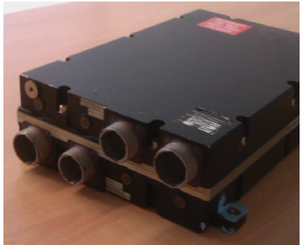
▲ Full-authority digital engine control unit
