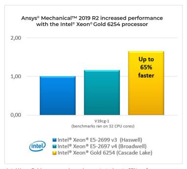
Intel Xeon Gold processors have demonstrated up to 65% performance increase on the geometric mean of 10 Ansys Mechanical benchmarks over the Intel Xeon E5v3 processor family.
