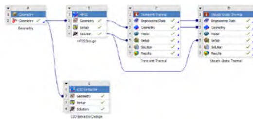
▲ ANSYS Workbench workflow for this multiphysics simulation
