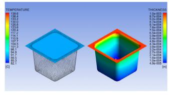
Homogenous temperature profile (left) and resulting wall thickness distribution (right) for a simple test cup.
