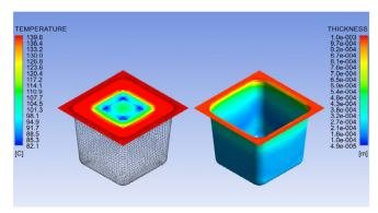
Optimized temperature profile (left) and resulting wall thickness distribution (right) for a simple test cup
