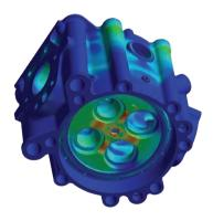
▲ Von Mises stresses caused by temperature and pressure on block
