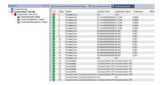
At test execution, SCADE Test Environment for Host automatically produces a test conformance report comparing actual results and expected results on host. This report includes a summary for quickly checking test status (Passed or Failed) along with further details to localize and understand issues.
