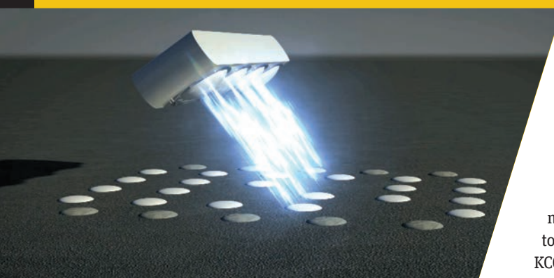
Four-radar RPS reading paint dot bit pattern on road
