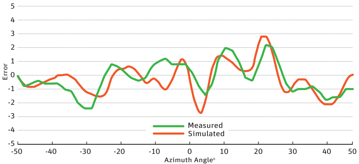
Predicted versus measured radar sensor bearing prediction error
