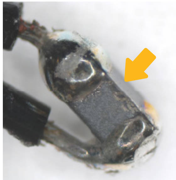
Thermistor post-decapsulation under optical microscope
